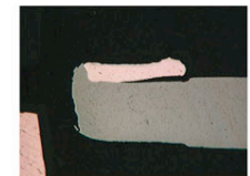
Poor Anode Weld (Tantalum Capacitor)
