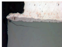
Cross Sectional View Of Diode Showing Fractures Die
